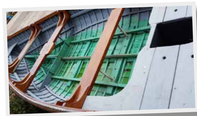
The last salmon coble built in Portrush by Billy Gregg. Note the well for an outboard engine. Courtesy Capt. Robert Anderson
