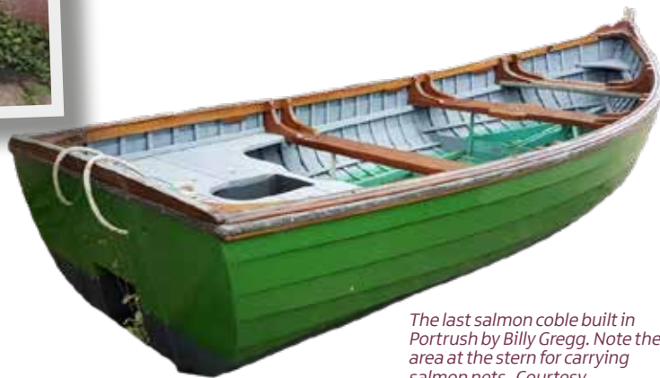
The last salmon coble built in Portrush by Billy Gregg. Note the well for an outboard engine. Courtesy Capt. Robert Anderson
