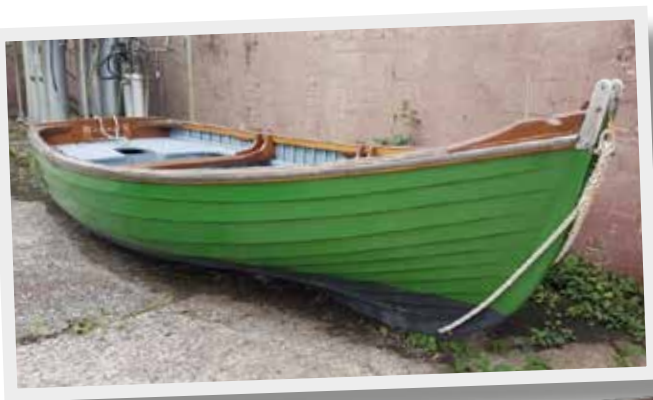
The bow of the last salmon coble built in Portrush by Billy Gregg. Though the stern differs, not being a 'double-ended' boat due to the need to pay nets out over the stern. The boat has a serial number of A15482.
